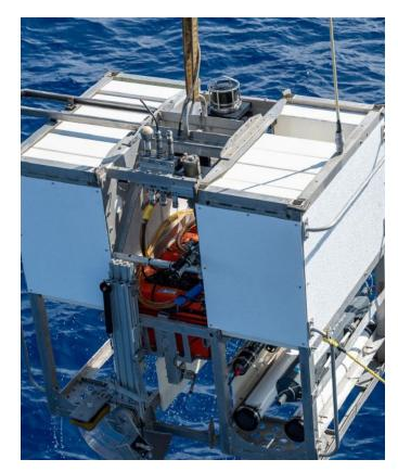
Figure 2: Deep dive of the new AquapHOx deep sea logger with the new optical pH sensor for the total scale in the Hawaiian Islands. (Credit: Discover Our Oceans LLC)
